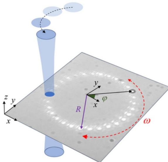
Figure 1. Schematic of a micro-bead (dark ring) driven over a landscape of optical traps (white spots).
