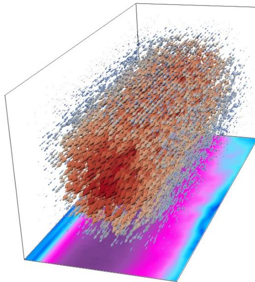
Figure 1. Flow and shear stress in a channel of an Organ-on-a-chip device
