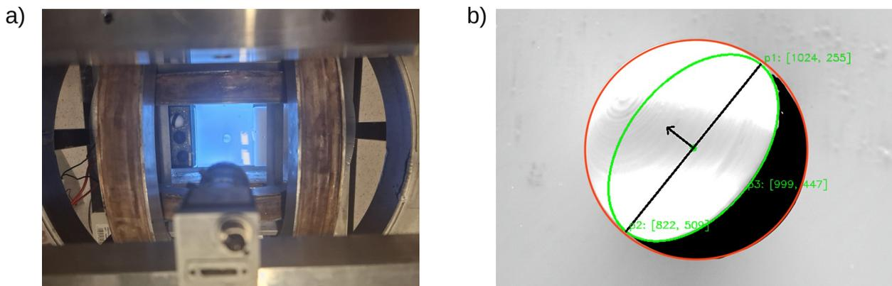
Figure 1. a) Experimental Apparatus; b) Magnetic Moment Vector Determination.
